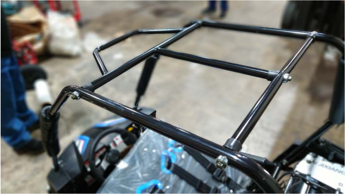
Figure 1.15: Install the Top Cross Bars
