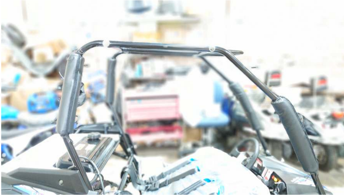
Figure 1.14: Install the Long Side Bars
