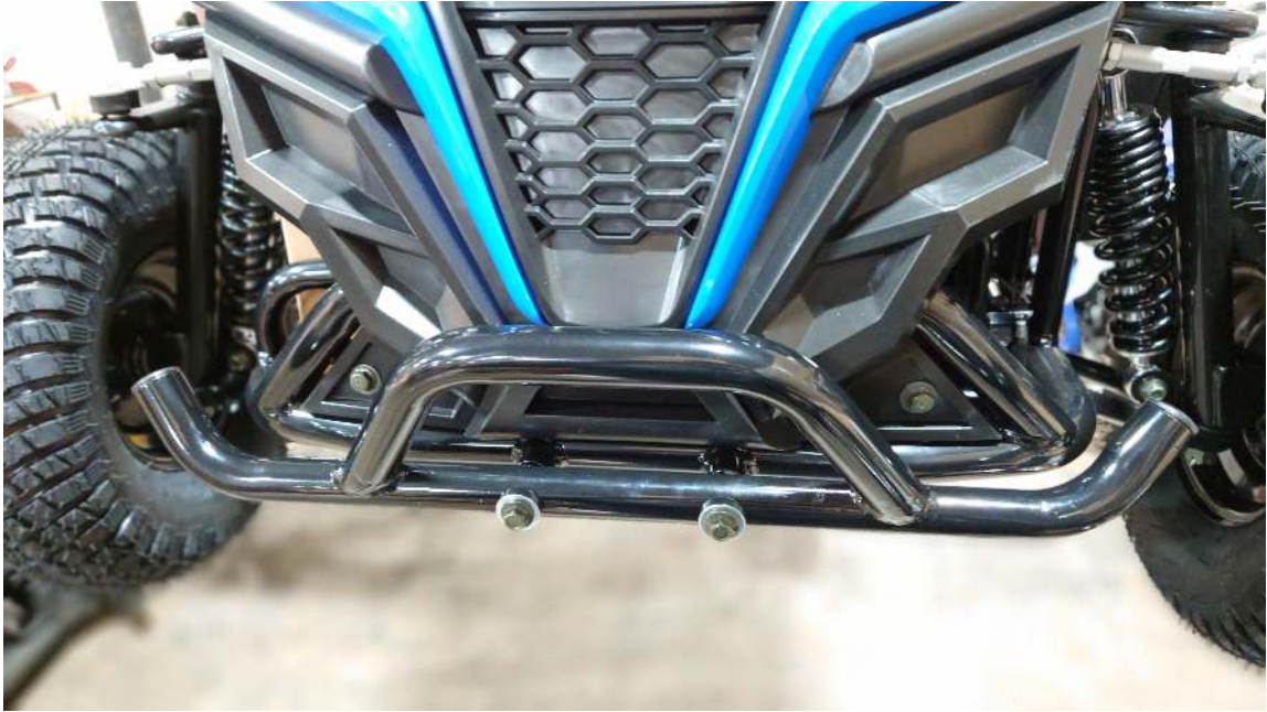
Figure 1.19: Install Protecting Bar
