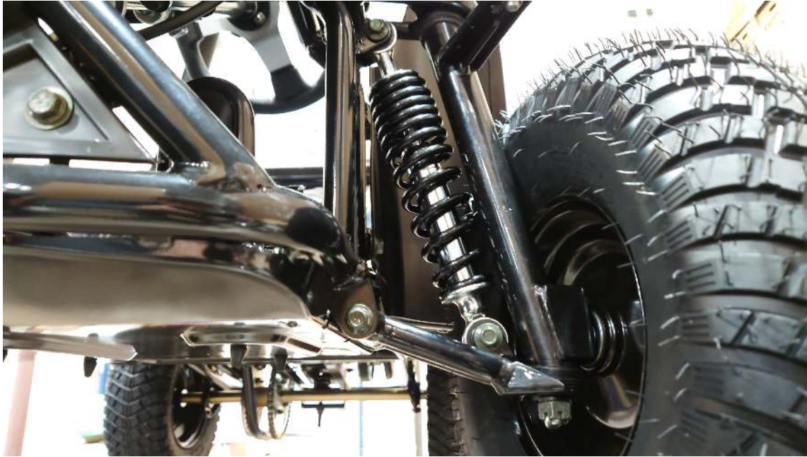
Figure 1.10: Install the Front Shocks and Spindles
