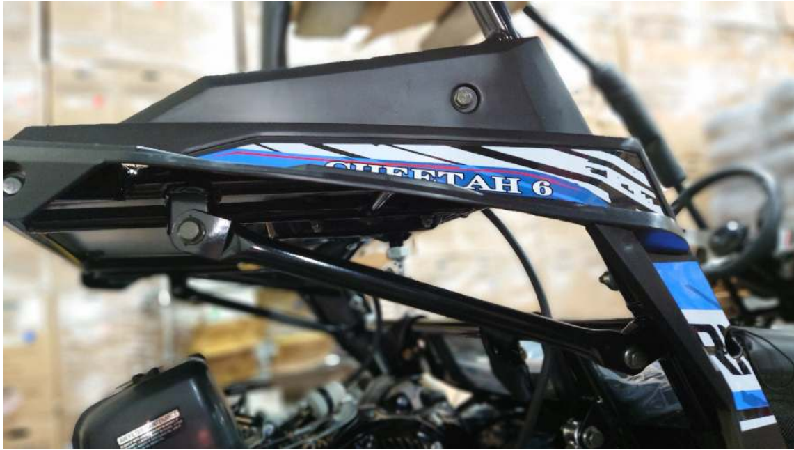
Figure 1.16: Install Rear Cage Rack and Cover
